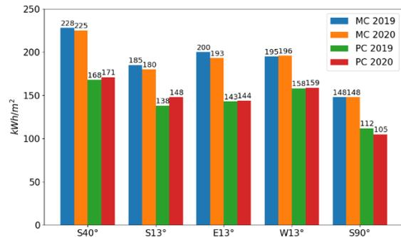
**Figure 2.** Total energy produced by varied-oriented panels during 2019 and 2020.
