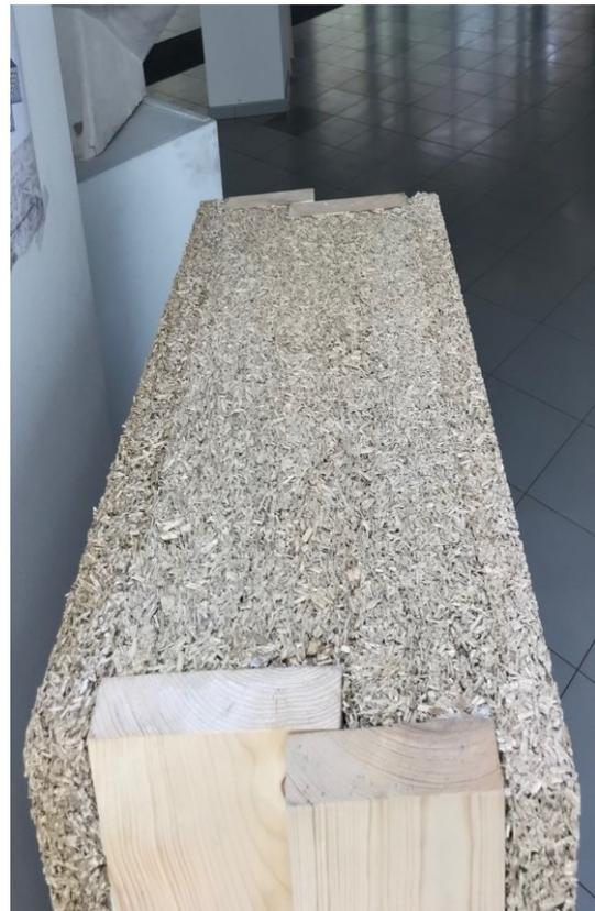
Figure 3. Experimental magnesium-hemp panel prototype.
