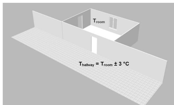
**Figure 5.3** *Relaxed thermal comfort requirements for transition spaces*
