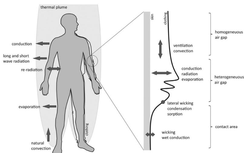
**Figure 5.1** The heat and mass transfer within the clothing system is a composition of a number of physical processes [1]
