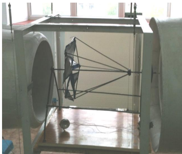
Fig. 7 The model of a sail type wind turbine in the test section of the T-I-M wind tunnel
