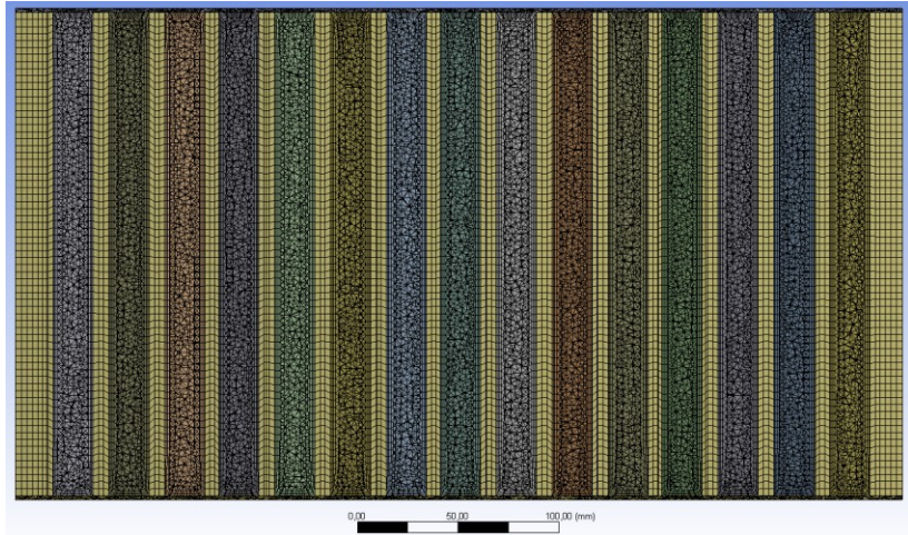
Fig. 3. Discretisation mesh in the middle cross-section of a modelled experimental block
